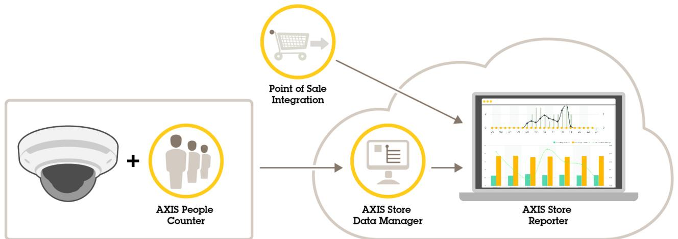
*An overview of the different devices, applications, and tools needed for a complete system.*
